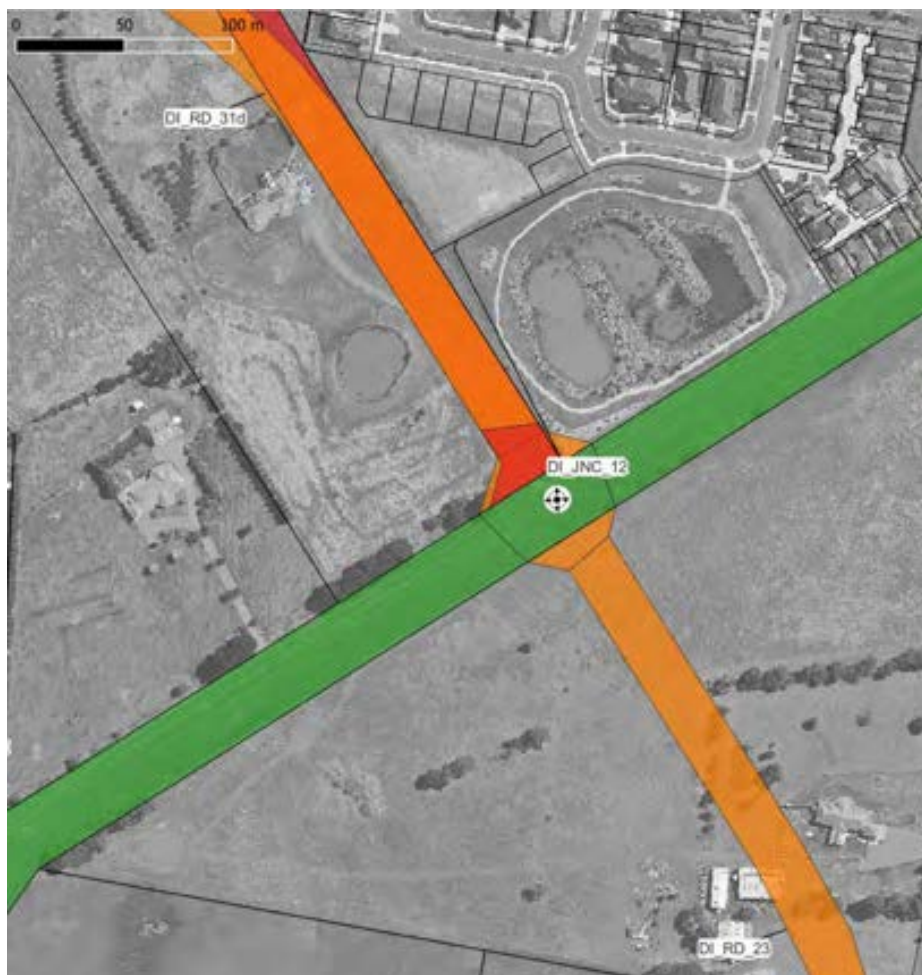
Figure 45 – DI_JNC_12 proposed alignment (orange), existing road reserve (green) and proposed re-alignment (red)
