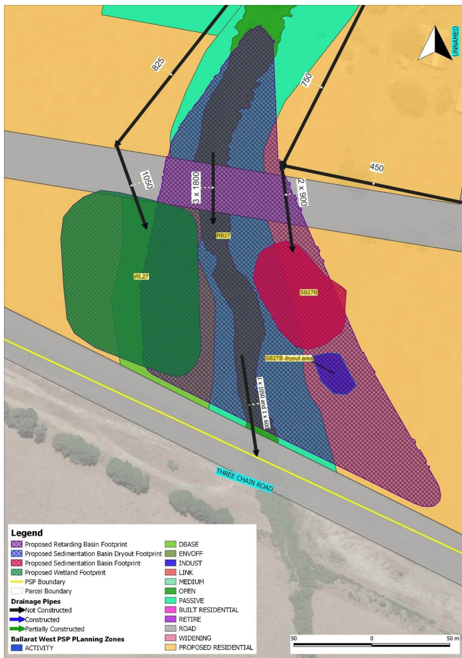
FIGURE 3.21: RETARDING BASIN 27 CONCEPT LAYOUT
