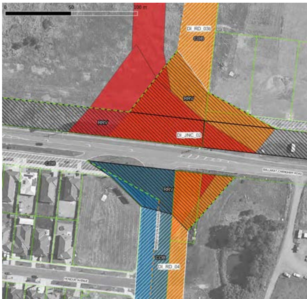
Figure 18 -Areas of responsibility (as hatching) of the proposed intersection of Carngham Road, Presentation Boulevard, Sydney Way
