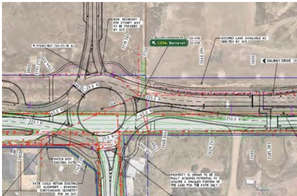
Figure 19 - DTP functional layout plan for two-lane roundabout (note pedestrian operated signals approx.200m east)
