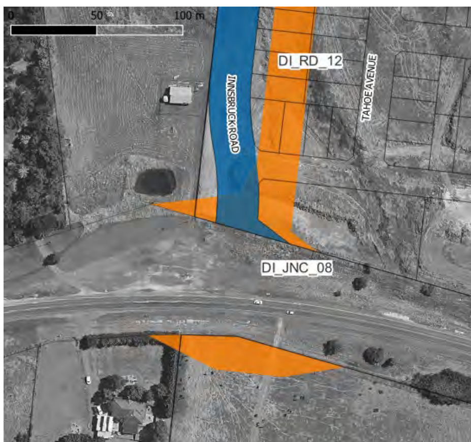
Figure 27 – Redesigned DI_JNC_12 (blue) and original alignment (orange)
