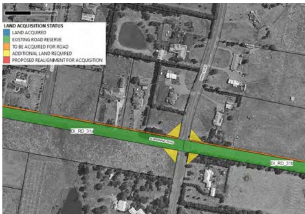
Figure 36 - Additional splays for DI_JNC_X1
