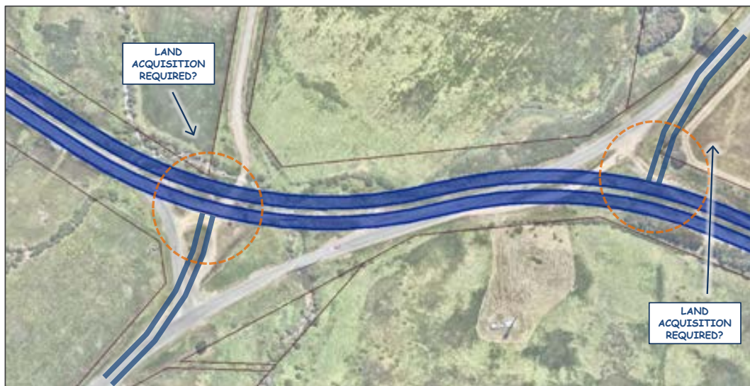
Figure 5.8 Ballarat Link Road Large Radius Alignment Sketch
