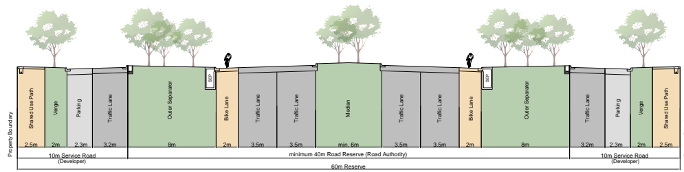
Figure 17: DLR2 - Duplicated Link Road with Service Road on both sides
