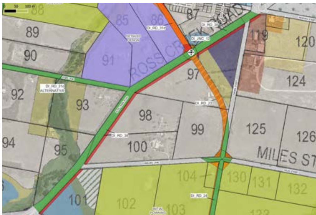
Figure 46 - properties where 10m is acquired for widened Ross Creek Road reserve (red) on the southern side.
