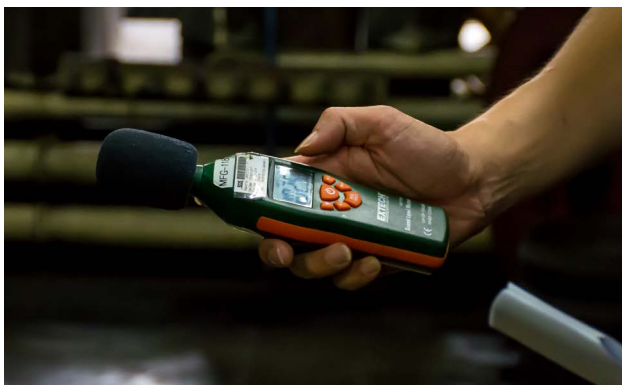
Checking sound levels
