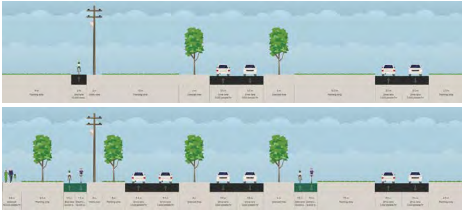
Figure 19 Remembrance Drive: Finchs Road to Link Road – Existing (top) and proposed (bottom)
