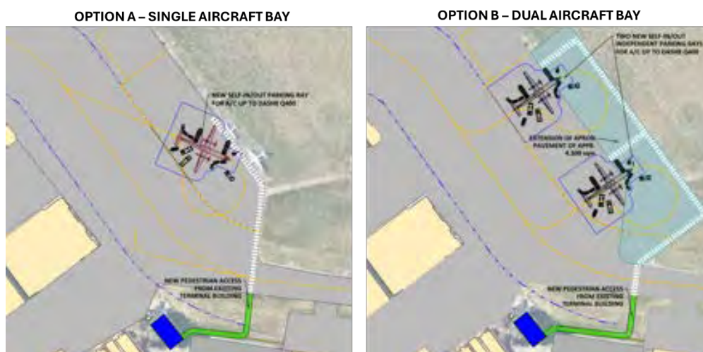
Figure 43: Existing Apron Area Redesign Concept Plan, Option A (left) and Option B (right)
