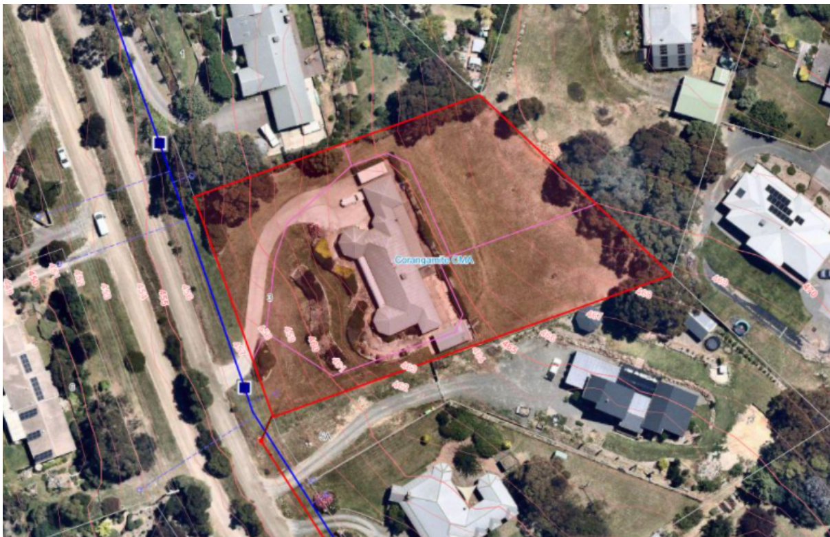
Image 4 – Aerial view, including sewerage (red) and potable water (blue). Source: IntraMaps
