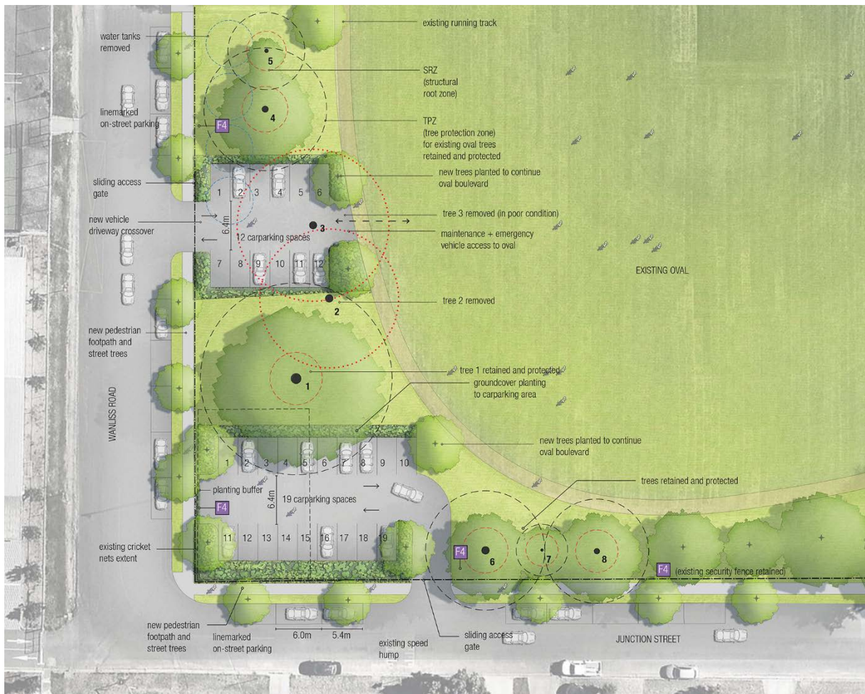
Figure 20: Proposed car parking spaces on-site and on-street along Wanliss Road and Junction Street
