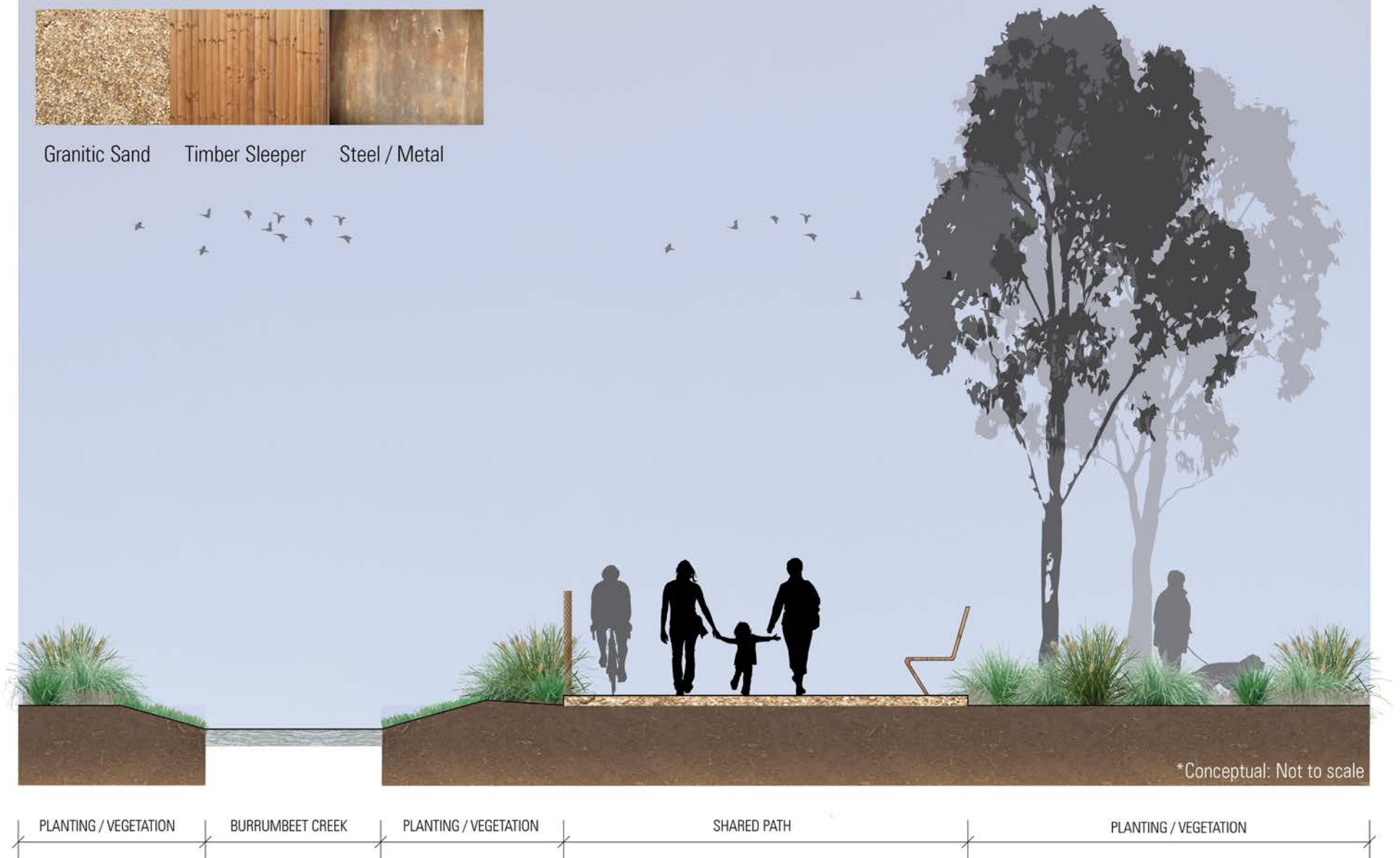
Figure 11 Conceptual section for potential shared path along Burrumbeet Creek
